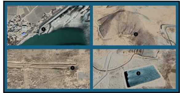
Figure 7 depicts an artificial water channel that carries water to the firing range from 35 km. The markings are explained as follows: 1. The diversion from the main Yarlung Tsan Po River; 2. The channel passes through the mountain via a tunnel; 3. The water is diverted and stored in an artificial pond; 4. The channel ends in the firing range—images Credits: Maxar & Google Earth.
