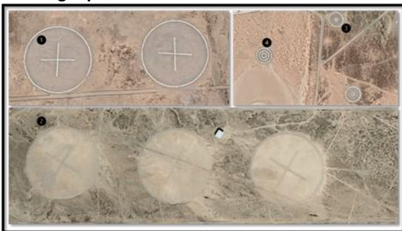
Figure 9 shows target pins of different sizes numbered as follows: 1. 50 m radius; 2. 100 m radius 3. 15 m radius with two concentric circles 4. 15-radius with three concentric circles, each with an interval of 5 m.
