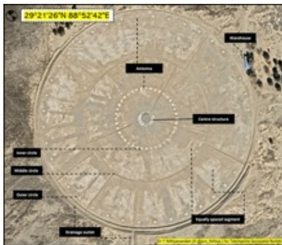
Figure 17 shows a massive circular feature related to signal intelligence. Images credit: Maxar & Google Earth
