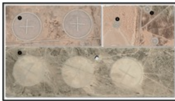
Figure 9 shows target pins of different sizes numbered as follows: 1. 50 m radius; 2. 100 m radius 3. 15 m radius with two concentric circles 4. 15-radius with three concentric circles, each with an interval of 5 m. Images credit: Maxar & Google Earth.
